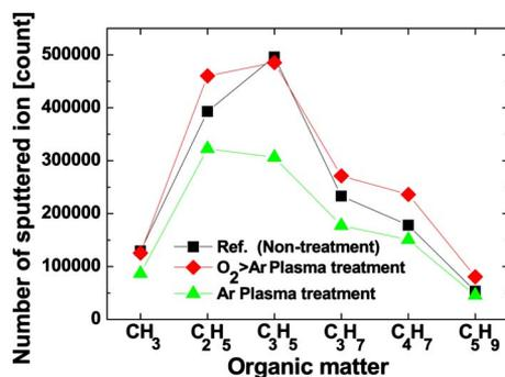
FIG. 2. (Color online) Comparison of organic matter ( $\text{C}_x\text{H}_y$ ) on MgO surface based on TOF-SIMS analysis of 50 in. full-HD panels prepared using rf-plasma treatment with various gas compositions.
