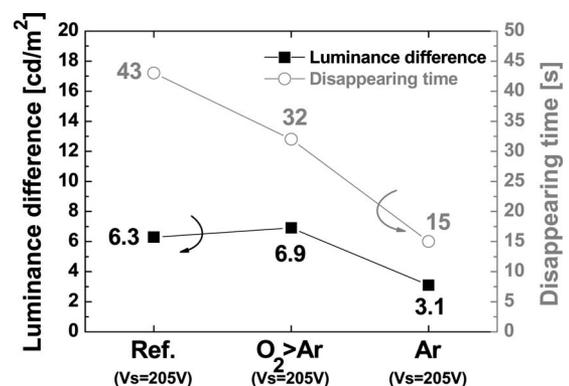
FIG. 3. Comparison of luminance difference and disappearing time of temporal image sticking with full-white background before and after 5 min. iterant sustain discharge in 50 inch full-HD panels prepared using rf-plasma treatment with various gas compositions.
