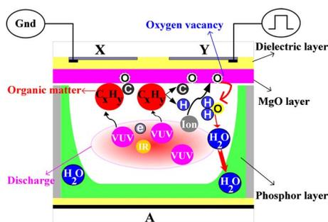
FIG. 1. (Color online) Mechanism inducing temporal image sticking in ac plasma display panel.
