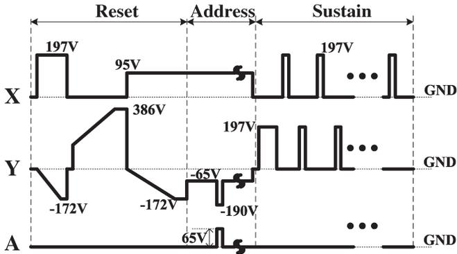
Fig. 2. Schematic diagram of driving waveform used in this study.
