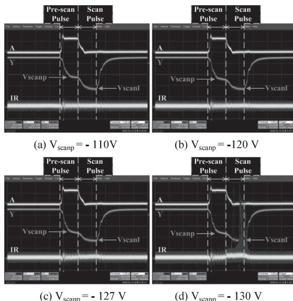
**Fig. 9** IR waveforms relative to  $V_{scanp}$  level during application of address pulse.
