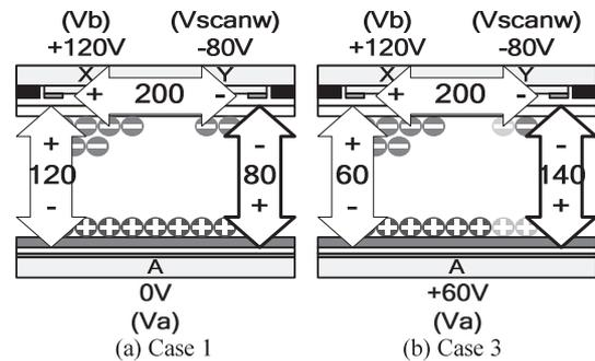
**Fig. 6** Voltage differences among three electrodes X, Y, and A experienced at  $A_j$ th cell in 768th scan line during line-by-line scanning from 1st to 767th line in address-period for two test patterns: (a) full-black test pattern (case 1), and (b) full-white test pattern (case 3).
