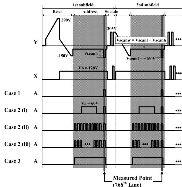
**Fig. 3** Driving waveforms employed to display five test patterns of Fig. 2.
