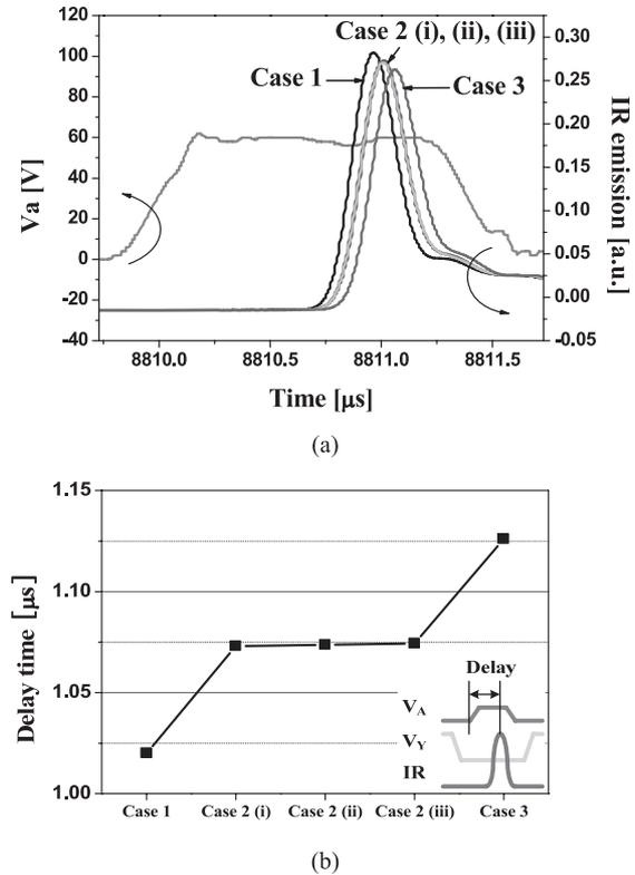
**Fig. 4** (a) IR waveforms emitted during address discharge at  $A_j$ th cell in 768th line relative to cases 1, 2 (i), (ii), (iii), and 3 in Fig. 2, and (b) corresponding address delay times.
