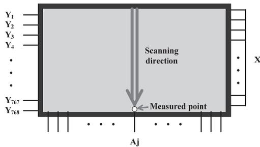
**Fig. 1** HD grade PDP with three electrodes where  $X$  is common (sustain) electrode,  $Y$  is scan electrode separated from  $Y_1$  to  $Y_{768}$ , and  $A$  is address electrode. Arrow seen above indicates scanning direction, and measured cell is located at last ( $=Y_{768}$ ) scan linen and at  $A_j$ th addresses line.
