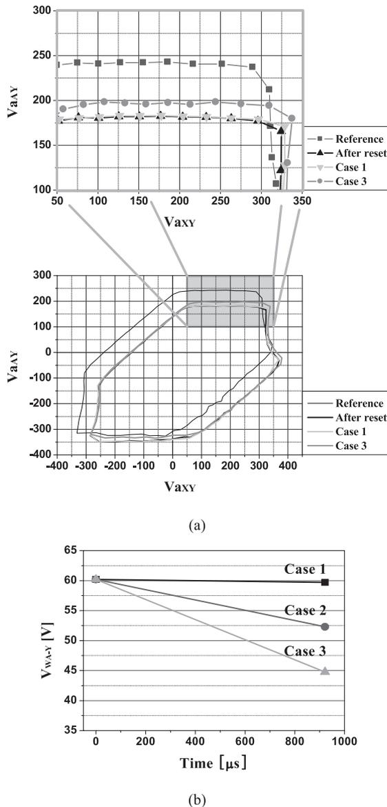
**Fig. 5** (a)  $V_t$  closed curves measured for full-black (case 1) and full-white (case 3) test patterns with respect to wall voltage state after rest-period where reference means zero wall voltage condition, and (b) variations in wall voltages between A-Y electrodes during address period for three cases 1, 2, and 3.
