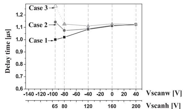
**Fig. 7** Changes in address delay time relative to variation of  $V_{scanw}$  ( $= V_{scanl} + V_{scanh}$ ) for different address-on-times (cases 1, 2, and 3).
