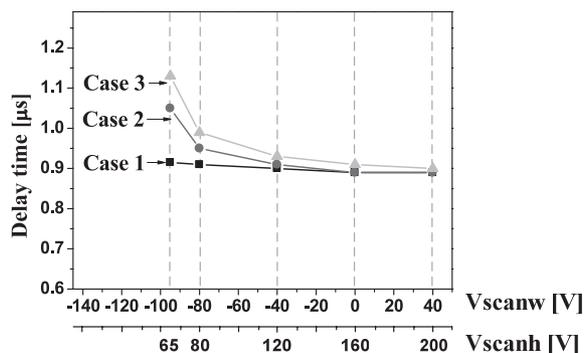
**Fig. 10** Delay time relative to cases of previous discharge time on address electrode when double scan pulse applied.
