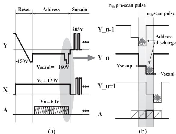
**Fig. 8** (a) Driving waveform with proposed double scan pulse consisting of pre-scan and scan pulses, and (b) enlarged double scan pulse applied from  $(n - 1)$ th to  $(n + 1)$ th scan line.
