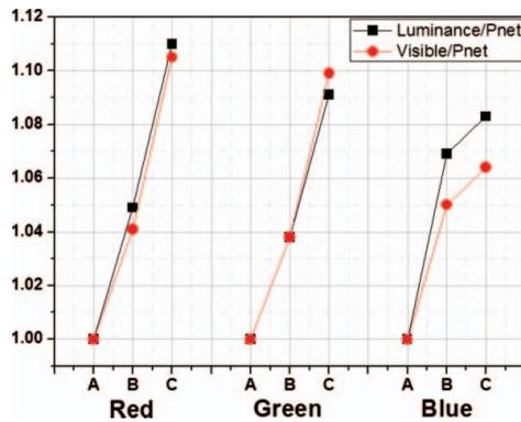
**Figure 7.** Comparison of luminance and visible light spectrum (400 nm ~ 750 nm) under various thicknesses of R, G, and B phosphor layer.
