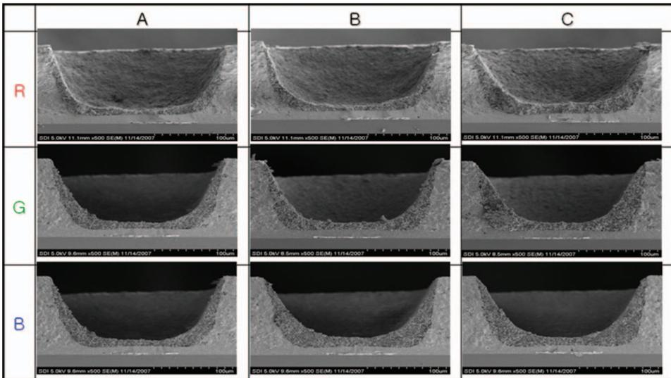
Figure 6. SEM images by thicknesses of red, green, and blue phosphor layers.
